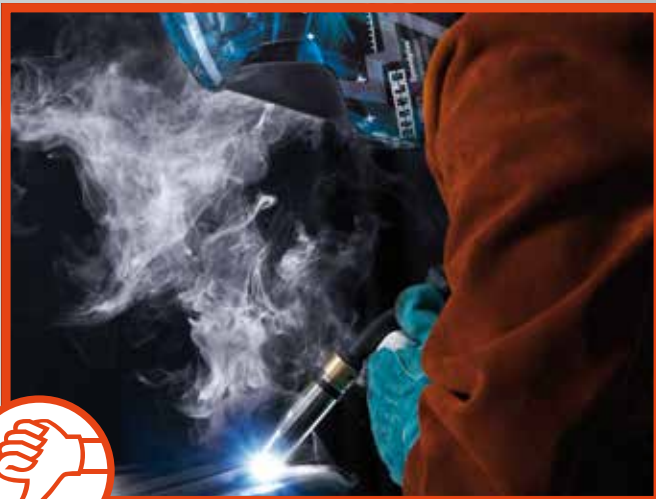
Standard welding torch: strong fume production!
